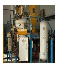
Metals and alloys that have a high affinity for gases, in particular nitrogen and oxygen are often melted/refined in vacuum induction furnaces to prevent contamination/reaction with these gases. Thus, the process is generally used for processing of high purity materials or materials with tight tolerances on chemical composition.
